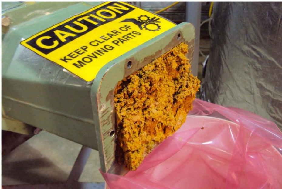
Figure 4 Mixture Exiting Extrusion Head Prior to blocking up with 5 th batch.
