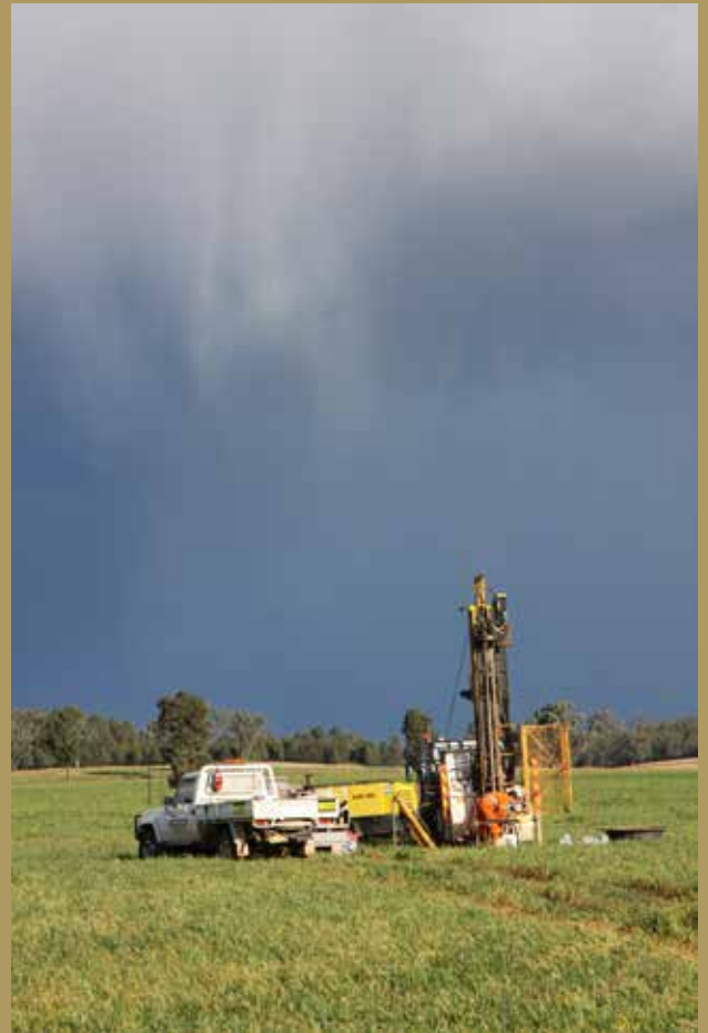
Light truck-mounted geotech diamond drill rig
