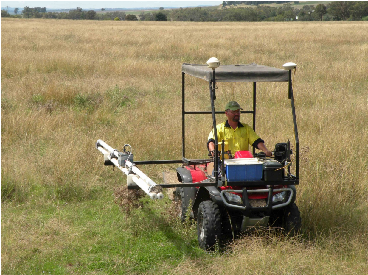
Plate 1 EM Survey Equipment. EM 31 is on frame beside operator, EM 38 is on conveyor belt dragged behind 4 wheel bike.
