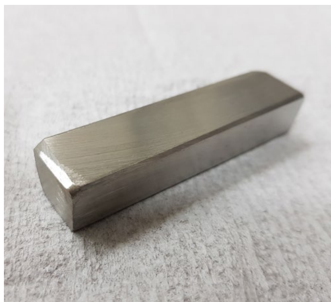
Neodymium-praseodymium alloy produced on the metallisation pilot plant
