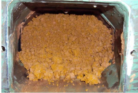
Figure 3 Filter cake after first pass through, with Rotary Blades and Extrusion Head.
